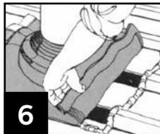
6 Apply a generous bead of neutral cure 100% silicone sealant (roof and gutter approved) to the underside of Dektite Soaker base along entire perimeter.
