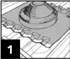
1 Mark position of pipe on roofing sheet, centre Dektite Soaker over mark ensuring word "top" is towards highest part of roof, and form Dektite Soaker flanges to roof profile.
