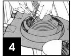
4 Trim Dektite Soaker cone to suit pipe size with sharp tin snips and slide down pipe using water as lubricant.
