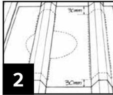
2 Mark ribs or corrugations to be removed to allow adequate drainage around cone. Allow at least 30mm all round to fasten Dektite Soaker's aluminium strips to roofing sheet.
