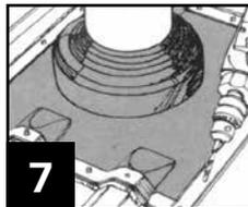
7 Fasten flashing to roof using washered self-drilling screws or sealed rivets, ensuring Dektite Soaker forms flat trough for water run-off. Fix integral aluminium strips from centre outwards before attaching loose strips provided.
