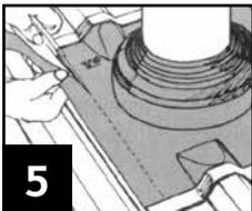
5 Form Dektite Soaker base into contours of roofing sheet, positioning loose strips on either side of cone in best position to ensure drainage of pan or tray. Trim excess EPDM from outside of loose strips. Trimming should be considered prior to cutting of the roof sheet.
