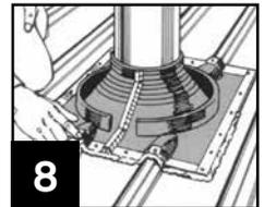
8 Apply neutral cure 100% silicone sealant (roof and gutter approved) to the top of crimp closure and any other potential leak areas.
