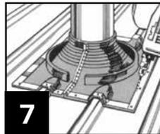
7 Fasten flashing to roof using washed self drilling screws or sealed rivets. Secure clip by placing a fastener either side of the clip. Fix integral aluminium strips from centre outwards before attaching loose strips provided.
