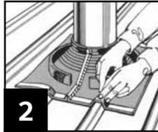
2 Mark out area where ribs of roof panel are to be removed. Where necessary support cut sections of sheet with additional roof framing.
