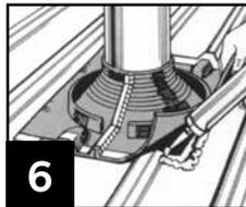
6 Apply a generous bead of neutral cure 100% silicone sealant (roof and gutter approved) to underside of Dektite base and press to contour of sheet profile.
