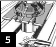
5 Form Dektite base into contours of roofing sheet, positioning loose strips on either side of cone in best position to ensure drainage of pan or tray and trim sides if necessary. Trimming should be considered prior to cutting of the roof sheet.
